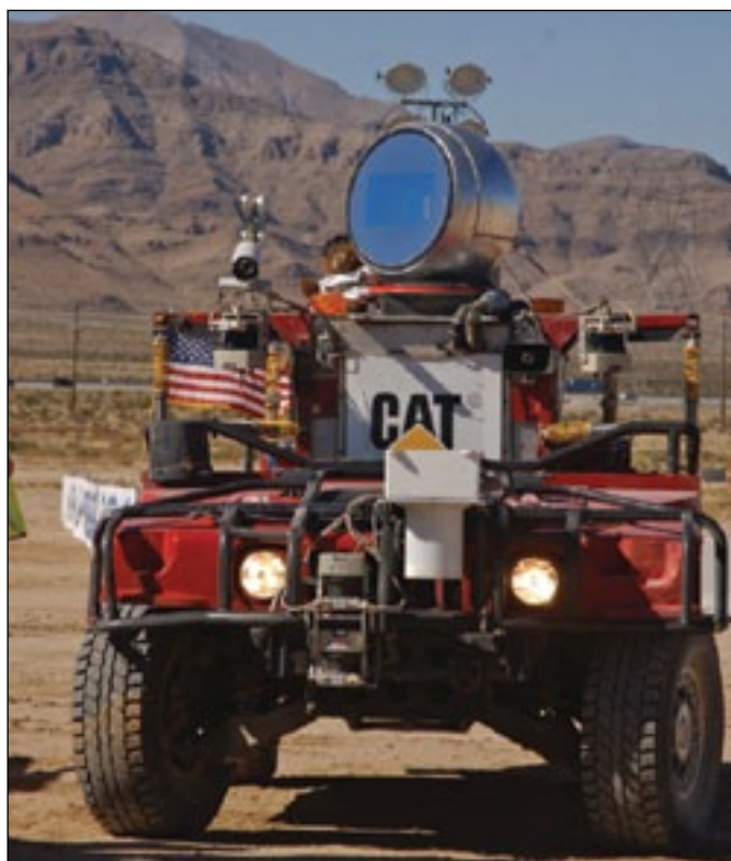
Contender in the 2005 DARPA grand challenge for autonomous ground vehicles
