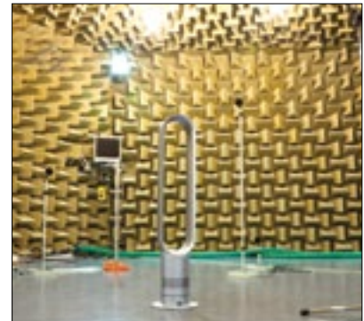
3. Testing the Dyson bladeless fan in the EMC Chamber
